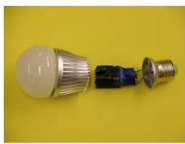
Efficient Lighting (LED driver)
